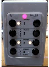
OFF—Fades output smoothly to off over 3 seconds, and deselects any active presets or RGB button combinations.
