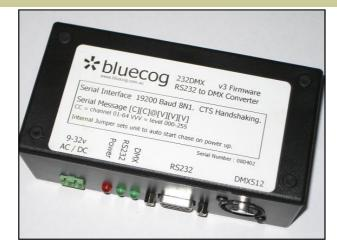
The bluecog RS232 to DMX interface box allows control systems and AV automation systems such as Crestron to control DMX based devices including LED lighting and moving lights.
